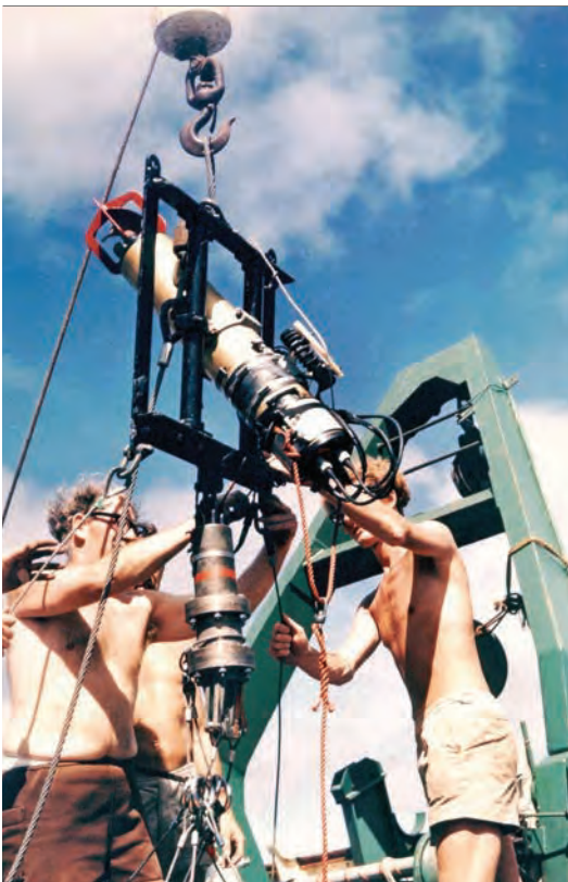
Howard Roe (right) and the author deploying the first monitor for the opening/closing net, designed and built by Derrick Bishop, Roy Bowers, Dicky Dobson and Malcolm Harris
