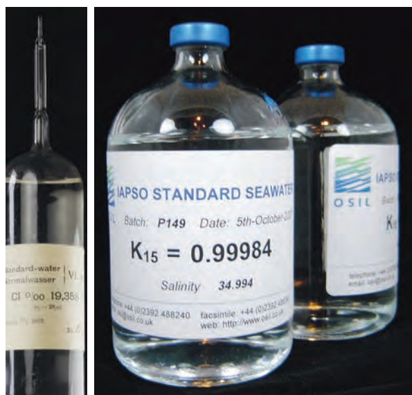
Left Close-up of an early ampoule of Standard Seawater calibrated in chlorinity.
