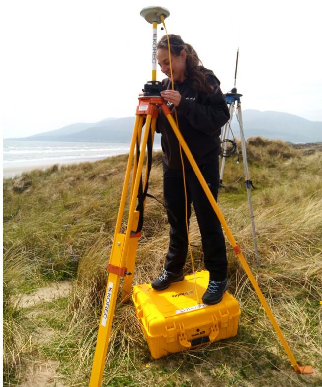
Dr Melanie Biousque of Ulster University is setting up a GPS surveying system as part of a beach monitoring programme at Dundrum Bay.
