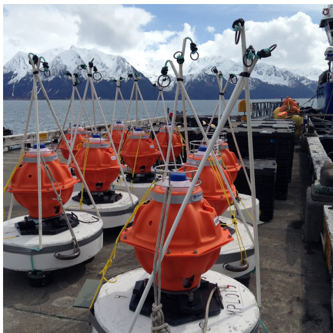
The seabed instruments which make up Sonardyne's seabed deformation monitoring system sit waiting to be deployed off the coast of Canada. Image credit: David Chadwell/ Scripps Institution of Oceanography
