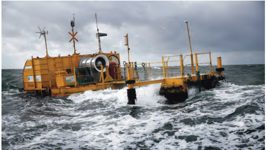
Ocean Energy Ltd from Ireland is planning to bring a full-scale version of its Ocean Energy Buoy to Wave Hub this year having tested this quarter-sized prototype for three years in Galway Bay.
