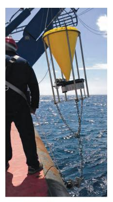
**Figure 4** A sediment trap being deployed at the PAP-SO site. The containers at the bottom move around every 2–4 weeks, allowing each in turn to receive material collected by the funnel, so providing an observational time-series.
