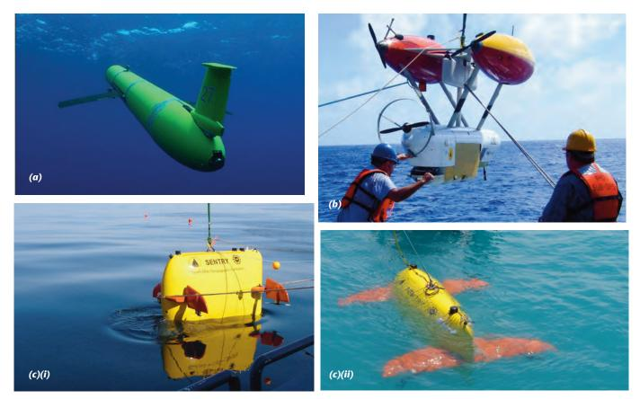
**Figure 2** Examples of some AUVs. (a) A Slocum buoyancy-driven glider. (b) Woods Hole's Autonomous Benthic Explorer (ABE), designed to investigate deep ocean environments such as hydrothermal vents. (c) ABE's successor, Sentry, (i) at the start of deployment, (ii) with its 'glider wings' extended. (Photos by courtesy of: (a) Rutgers University; (b) Dana Yoerger; © WHOI and (c) Chris German; © WHOI)
