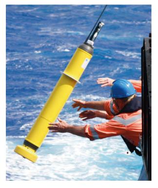
Figure 3 An Argo float being launched into the Indian Ocean (By courtesy of CSIRO) data are transmitted back to the shore laboratory.
