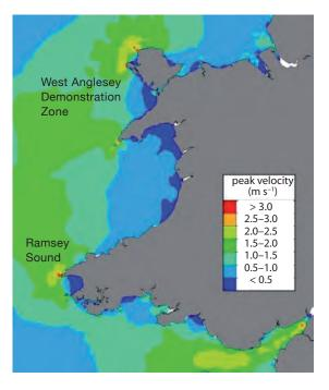
Figure 1 Hydrodynamic model showing the peak tidal velocities in the waters around Wales. The West Anglesey Demonstration Zone and Ramsey Sound are potential sites for tidal stream energy projects. (SEACAMS Research Office)
