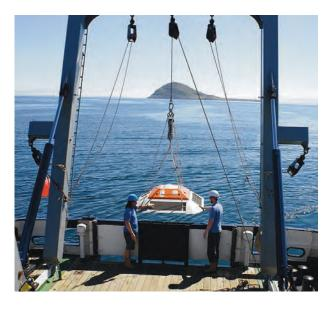
**Figure 2** An ADCP being lowered to the sea bed from the RV Prince Madog. This is part of the range of equipment made available to companies participating in SEACAMS.
