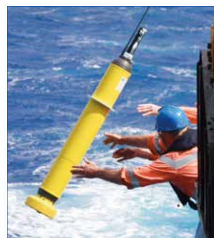
Launching an Argo float from Australia's RV Southern Surveyor. (Photo: Alicia Navidad, CSIRO)
