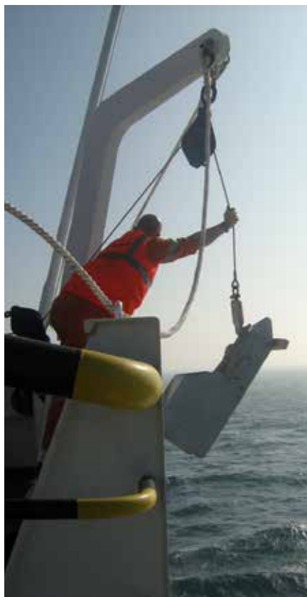
Figure 2 Left Deploying a Continuous Plankton Recorder (CPR) from a commercial vessel, so that it can be towed. Above A compilation of CPR tracks over the last 60 years. The white lines are routes in operation today, and pale blue lines are routes for which funding is being sought. The yellow line is the CPR route dedicated to collecting data for ICOS (footnote on p.17). (By courtesy of the Marine Biological Association)
