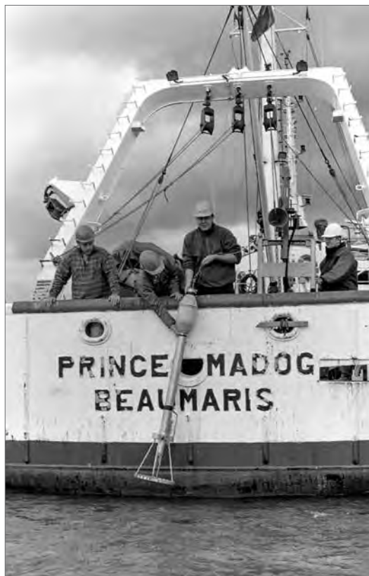
Figure 9 Tom Rippeth deploying a turbulence profiler, together with Mark Inall, Ray Wilton and Phil 'the bosun' Jones. The Prince Madog was used extensively to survey turbulence across the contrasting shelf-sea regimes around the UK. These measurements allowed the testing of state-of-the-art ocean models. (Photo: School of Ocean Sciences, Bangor University)
