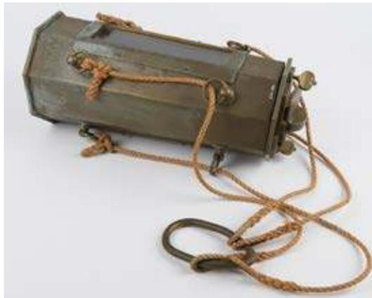
**A replica of the 'marine diver', based on Scoresby's description and drawing. The original was made in 1811 and lost in 1817 when the rope broke.**
