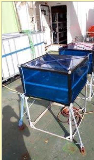
*On-deck incubators for bioassay experiments, where Lukas exposed the planktonic and microbial communities to an altered nutrient regime to mimic future conditions. To maintain a stable temperature, a continuous flow of seawater was supplied to the incubators, pumped up as the vessel was underway. (Photo: Lukas Marx)*
