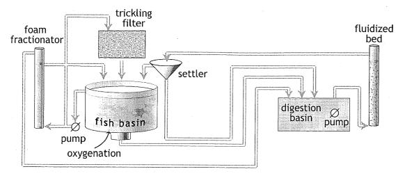
Figure 3 Schematic diagram of the recycling biofilter system (see also Figure 4).
